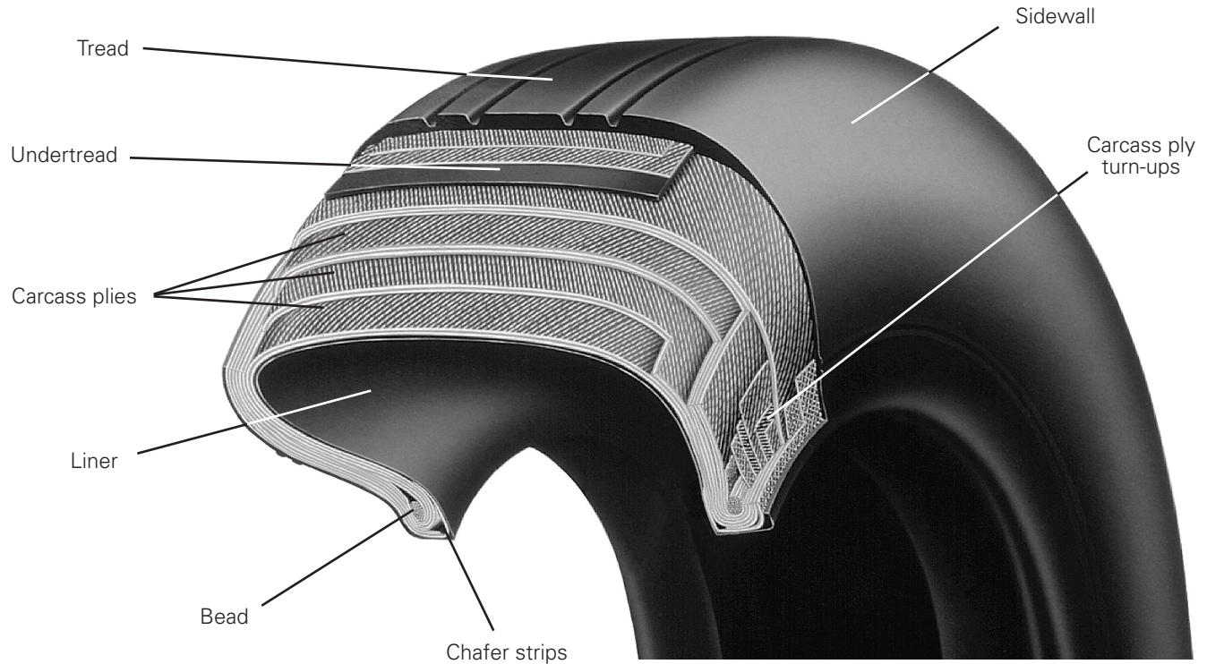
Typical bias-ply tire construction.
