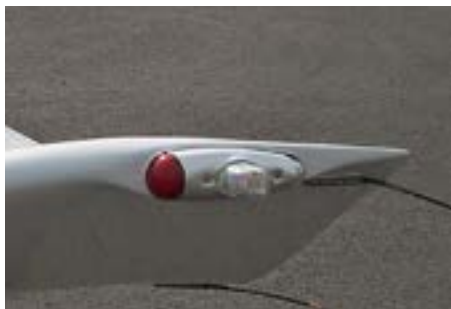
Legacy Strobe/Position light configuration
