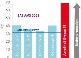
A step change in extreme-pressure protection. AeroShell Grease 58 has better load wear protection compared with MIL-PRF-81322 greases in ASTM D2596 tests.
