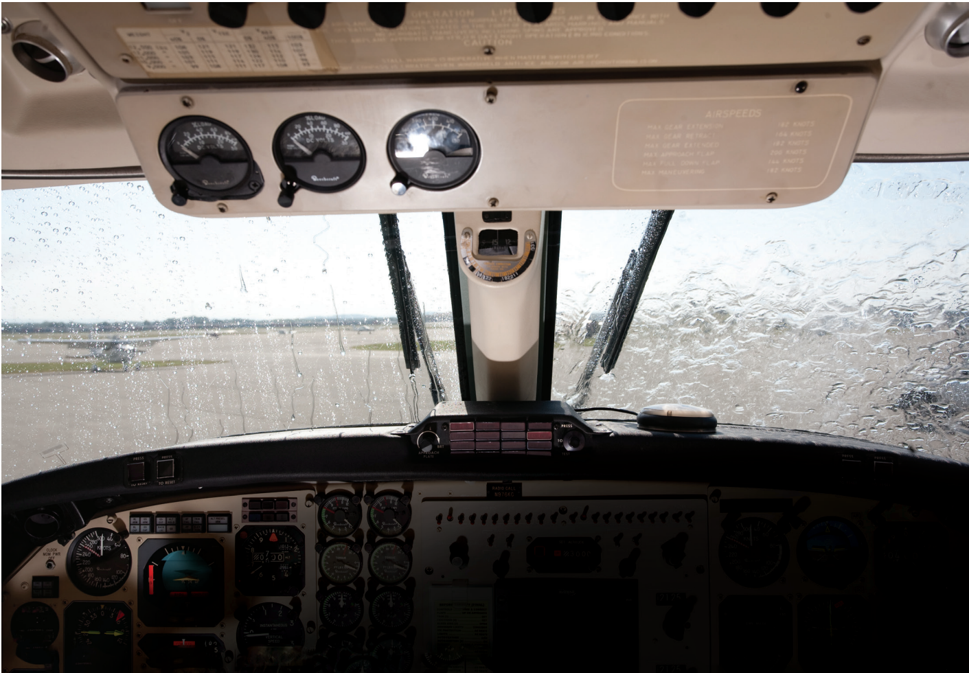
Surface Seal hydrophobic coating gives the pilot windshield (upper image left) enhanced visibility during wet conditions compared with the untreated co-pilot windshield (upper image right) as demonstrated by this simulation
