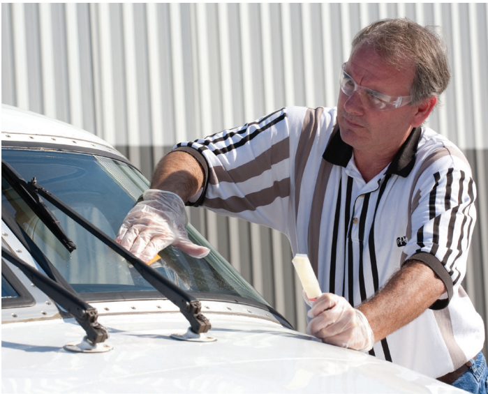
Surface Seal hydrophobic coating gives the pilot windshield (upper image left) enhanced visibility during wet conditions compared with the untreated co-pilot windshield (upper image right) as demonstrated by this simulation
