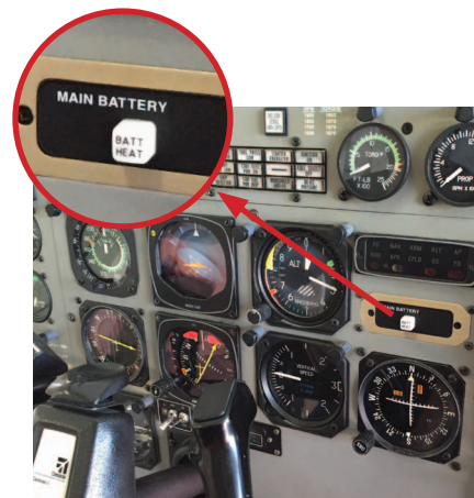
ACU installation has multiple approved placements on the instrument panel
