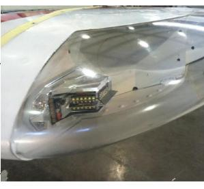
This Option includes removal of the OLD Grimes Strobe System and Installation of the Orion 650E per Whelen STC SA800EA
