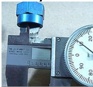
Measuring "B" nut thread size
