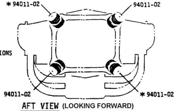
\* NOTE: WHEN 94011-02 AND 94011-20 ISOLATORS ARE USED TOGETHER, INSTALL 94011-20 AT THESE LOCATIONS.
