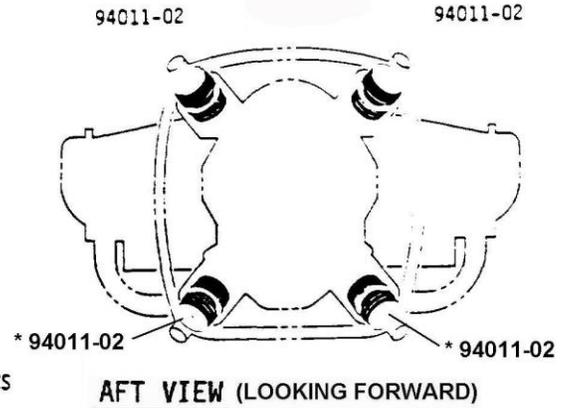
\* NOTE: WHEN 94011-02 & 94011-03 ISOLATORS ARE USED TOGETHER, INSTALL 94011-03 AT THESE LOCATIONS
