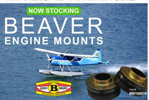
BARRY vibration isolation systems are used to mount the Pratt & Whitney R-985 and R-1340 engines in the aircraft and are designed to isolate powerplant vibrations from the airframe. Spring-rate and damping properties have been optimized to protect the pilot and aircraft structure from damaging vibration.
