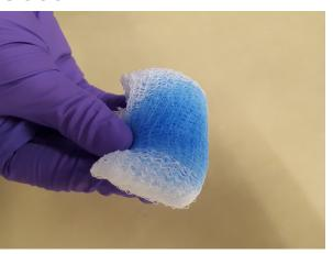
Lightly wet a clean gauze pad or AMS3819 wipe with the adhesion promoter. The gauze or pad should be moist, but not soaked or dripping wet.
