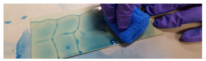
Apply a thin, uniform film to the surface of the substrate by wiping the substrate with the wetted gauze or pad. Adhesion promoter is not a paint or coating, it is not necessary to build up a certain thickness. A very thin layer, just enough to wet the surface, is all that is needed for the chemicals in the adhesion promoter to activate the surface for bonding.
