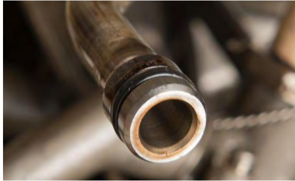
Sealing rings in excellent condition throughout, including this oil spray nozzle
