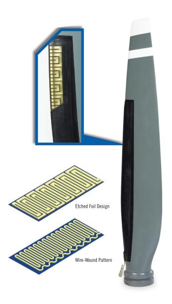
Ice Shield™ offers a diverse line of propeller boots for a variety of piston and turboprop aircraft in both wire-wound pattern and etched foil design. Whatever your propeller needs, you can feel confident that you are receiving a superior quality product from a company dedicated to your satisfaction.
