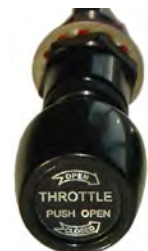
A vernier without a release button! See page 43
