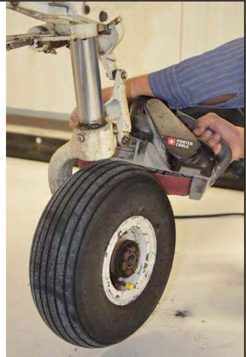
Use a belt sander to remove the shimmy wear pattern in the tread.
