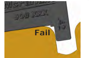
3. If the step touches the rail, lifting the gauge up, the wear is less than 0.42. If the step does not touch the rail, the wear is more than 0.42 and the seat rail must be replaced.
