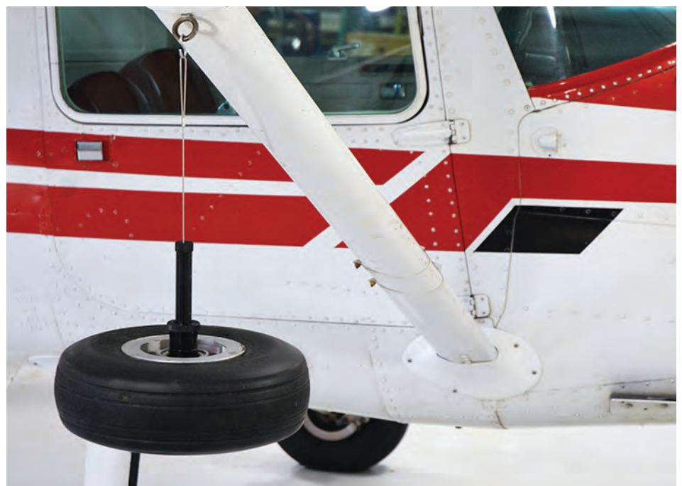
Use wheel balancer P/N TOOL128 for 3/4" diameter axles or P/N TOOL129 for 1", 1 1/4", and 1 1/2" axles to check tire for proper balance (additional sizes available). See page 242 for additional information.
