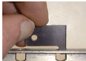
1. Place the gauge into each hole location showing wear.
